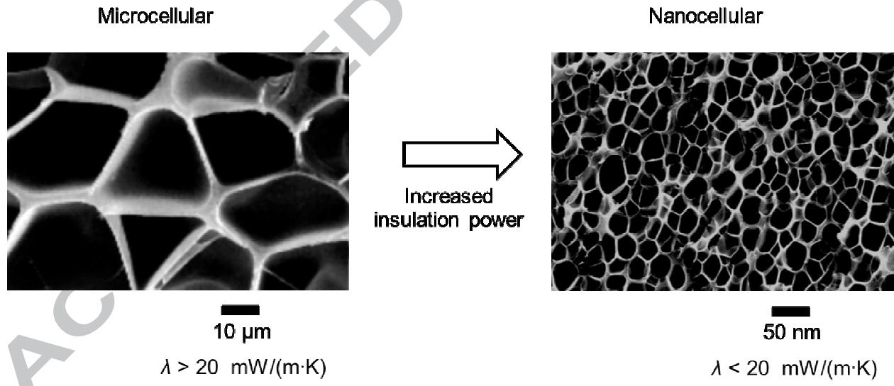
Keywords: Nanocellular polymers, cell nucleation, thermal conductivity, foam.
